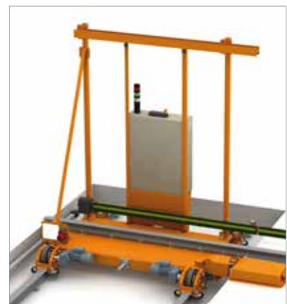
Details of a transfer bridge (2).
