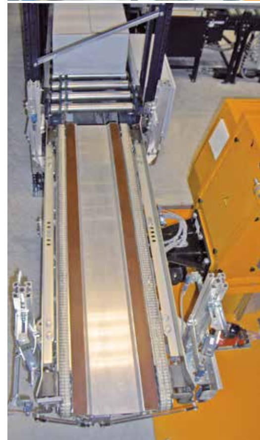
Details of the extraction system that combines forks with belts (EC).
