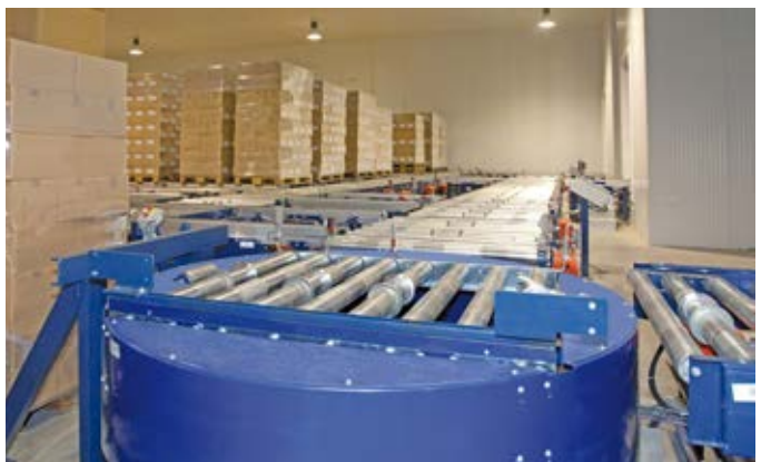
Mixed transfer with rollers and chains
