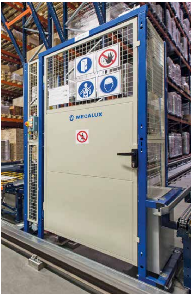
Control and maintenance zone partitions
